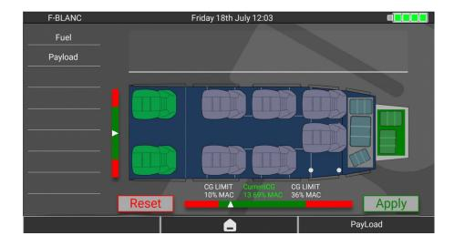
Each loaded passenger comes with their baggage allowance, which varies depending on whether you are in the base or cargo pod variant. The passenger baggage is loaded in the cabin baggage shelf and cargo pod, whereas the crew luggage is loaded in the aft luggage bin. Where applicable, loading happens fore-to-aft to maintain the center of gravity within limits.
