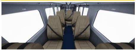
The empty cabin features a new loading system through the tablet. The user can select what type of cargo they want to load -i.e. crates, barrels- and click where they want to load them. Once the load is applied, the cargo weights are automatically applied to the aircraft.
