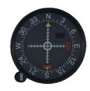
A knob at the 7 o' clock position will allow the pilot to rotate the course drum to the desired course, which will be at the top of the circle. The horizontal and vertical bars indicate glideslope and localizer deviation respectively. The instrument contains additional indications which are illustrated on the image below.
