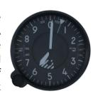
position in millibars. Three needles indicate the current altitude in 100ft (long needle), 1000ft (short needle) and 10000ft (thin needle
