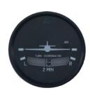
When the aircraft is in a slip, the ball will be off-centre in the direction of the turn. In practical turns this means that the plane is turning but the nose is pointing "outside the turn".
