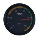
When the oil pressure is outside the green band, a red warning light labelled "OIL" will illuminate.
